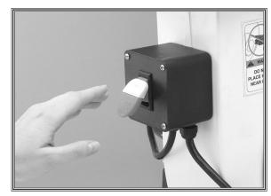
**Figure 24.** Hand position for emergency stop.
